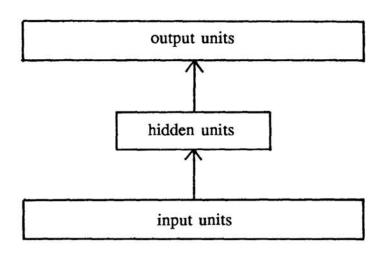
Fig. 1. A diagram of a three layer encoder network that learns good codes using back-propagation. On the forward pass, activity flows from the input units in the bottom layer to the output units in the top layer. On the backward pass, errorderivatives flow from the top layer to the bottom layer.
