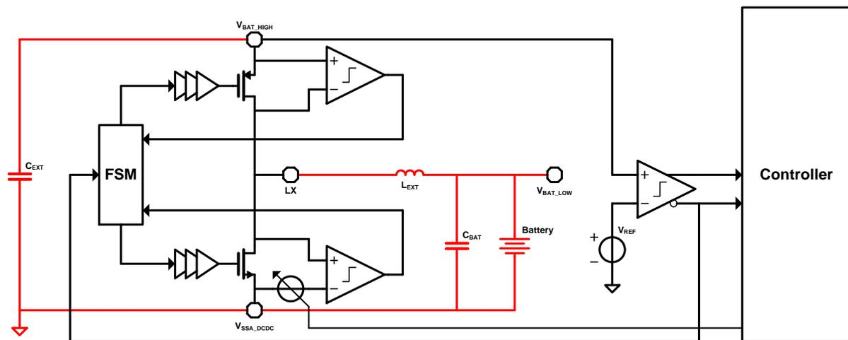
Figure 75: DCDC Block Diagram - Boost Configuration
