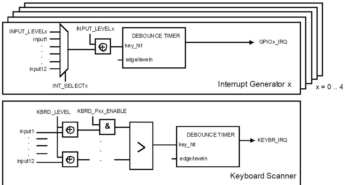
Figure 65: Keyboard Controller Block Diagram
