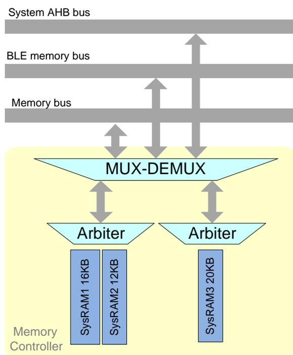
**Figure 25: Memory Controller Block Diagram**
