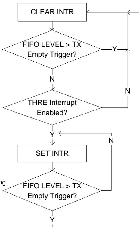
Figure 47: Flowchart of Interrupt Generation for Programmable THRE Interrupt Mode
