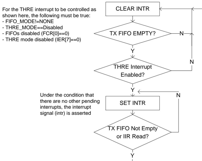
**Figure 48: Flowchart of Interrupt Generation When Not in Programmable THRE Interrupt Mode**
