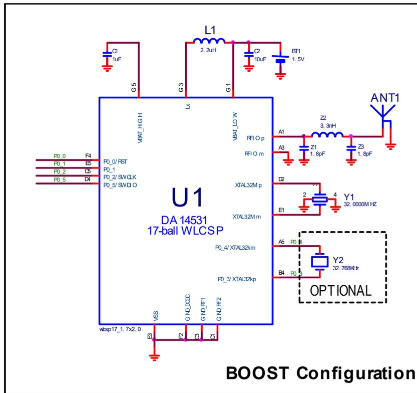
Figure 5: Boost Configuration System Diagram
