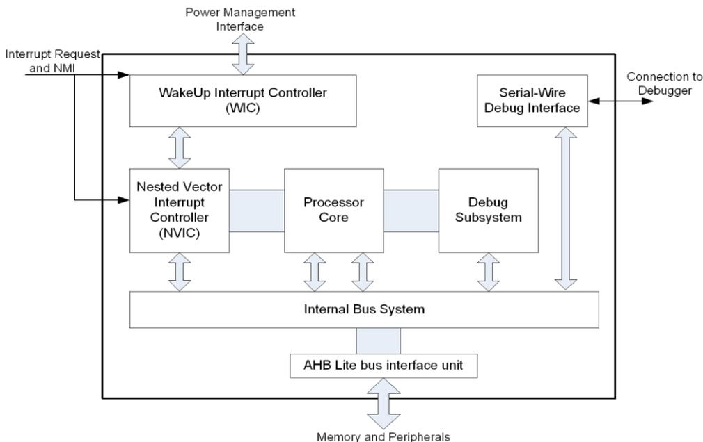
**Figure 23: Arm Cortex-M0+ Block Diagram**
