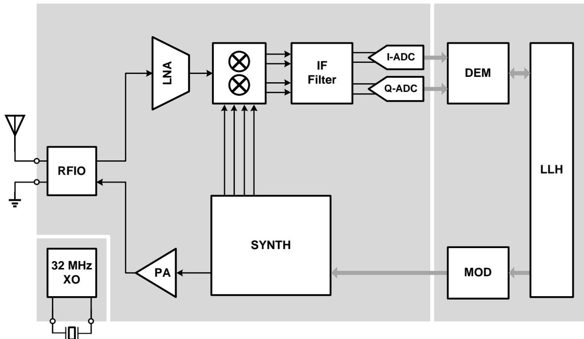
Figure 84: Bluetooth® Radio Block Diagram
