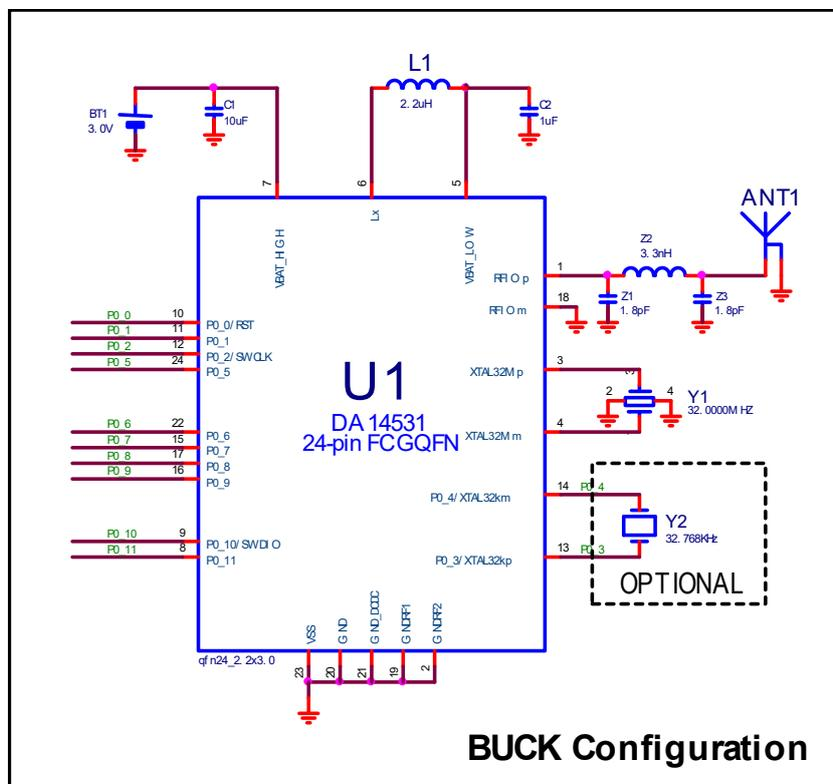
Figure 6: Buck Configuration System Diagram
