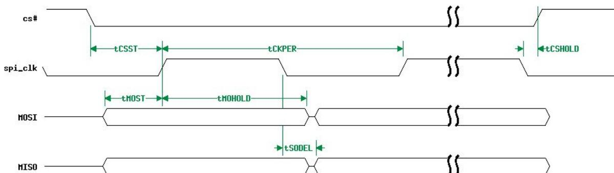
**Figure 50: SPI Slave Mode Timing (CPOL = 0, CPHA = 0)**
