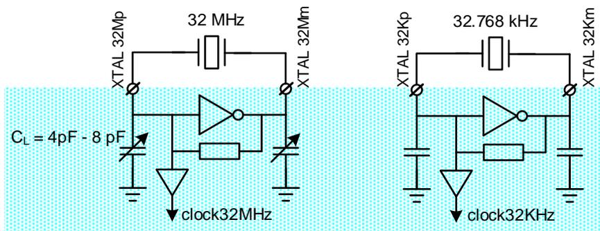
Figure 27: Crystal Oscillator Circuits
