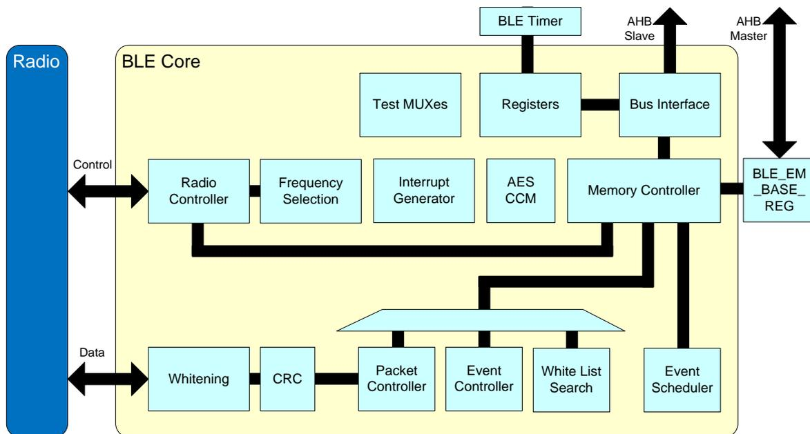
**Figure 78: Bluetooth® LE Core Block Diagram**
