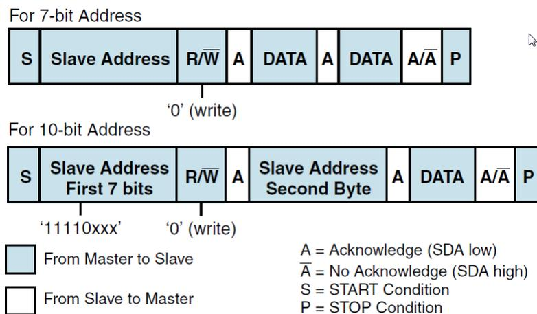
**Figure 39: Master-Transmitter Protocol**
