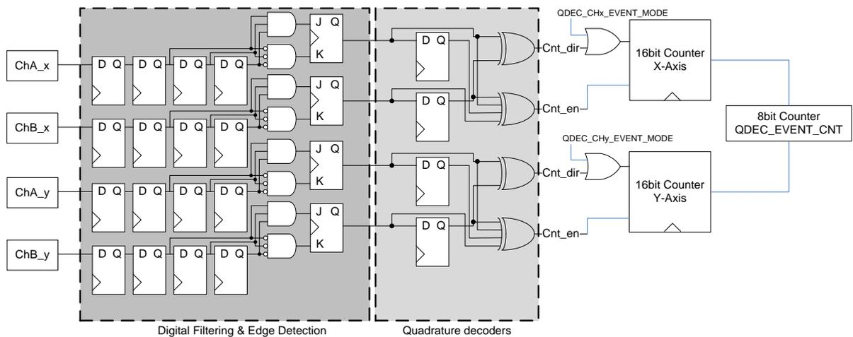
Figure 54: Digital Filtering and Edge Detection Circuit
