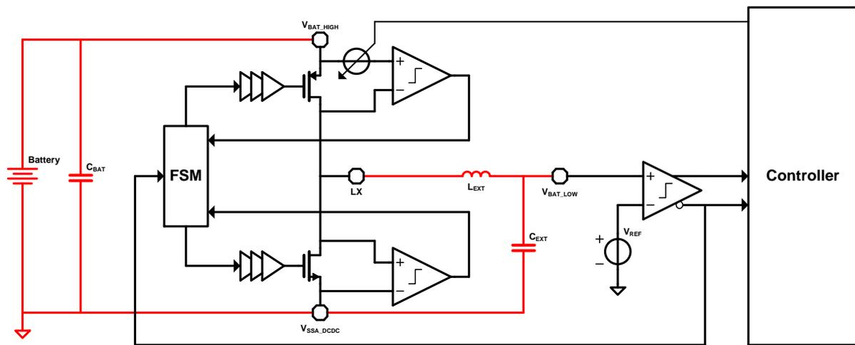
Figure 74: DCDC Block Diagram - Buck Configuration
