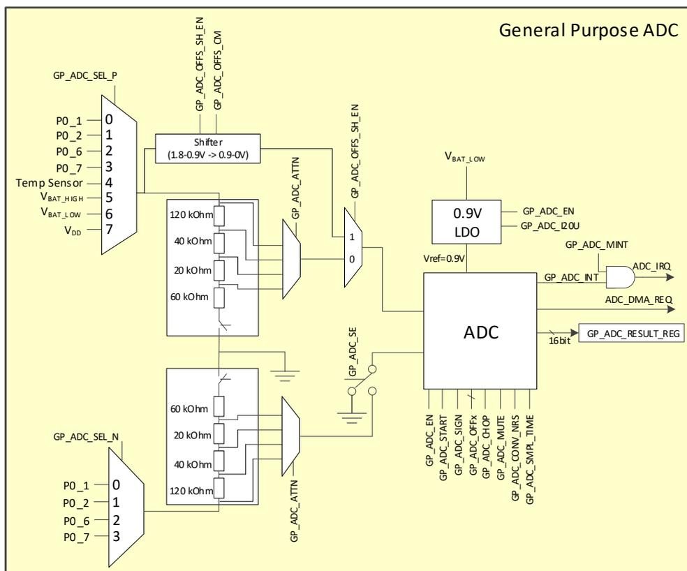
Figure 71: Block Diagram of GPADC
