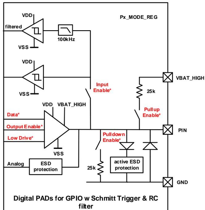
Figure 70: Type B GPIO Pad - GPIO with Schmitt Trigger and RC Filter on Input
